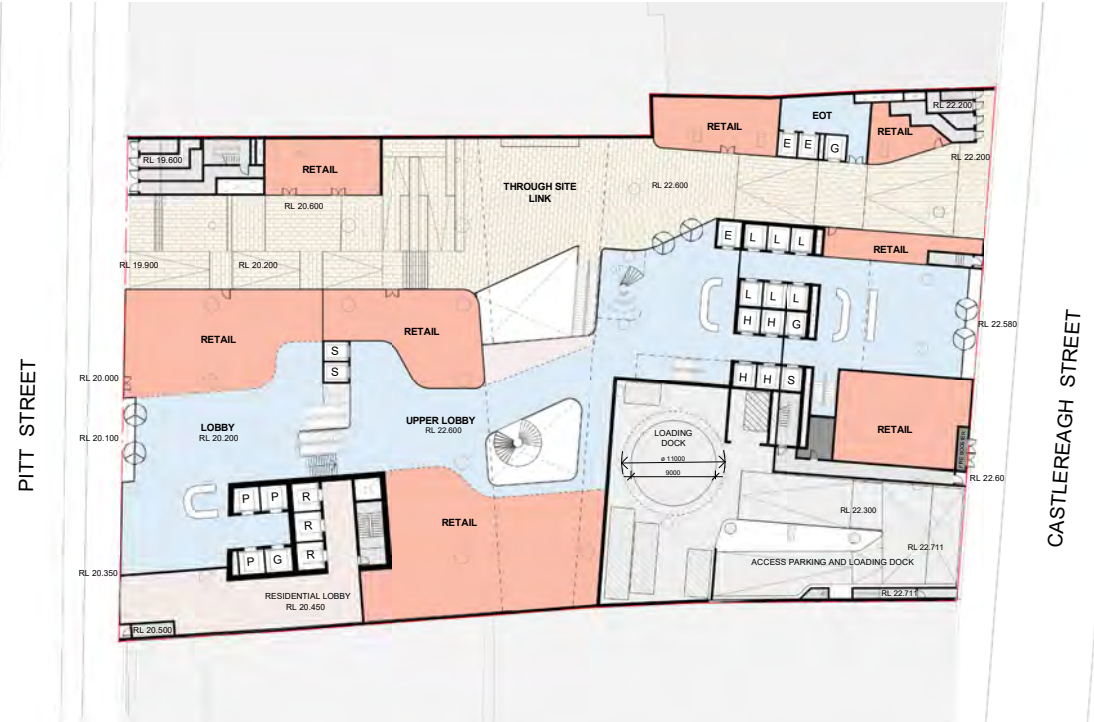
Ground - MRV and SRV Loading Dock
